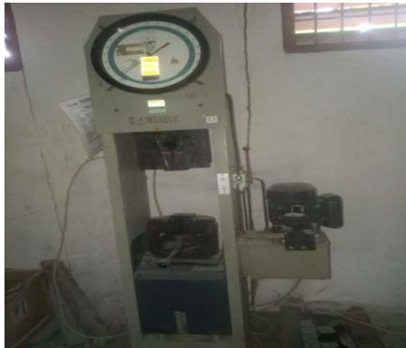
Gambar 3.1 Universal Testing Mechine (UTM). Jenis Load Cell , daya.3000 kN merk MATEST ITALY
