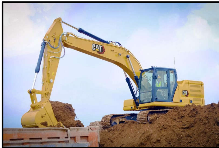
Gambar 2. 1 Alat Gali Muat Excavator (CAT 320 TIER 3 2021)
