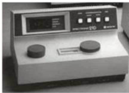
Gambar 2.3 Spektrofotometer UV-Vis Single-beam (Spectronic 21)
