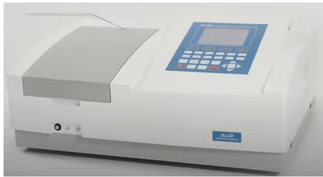
Gambar 2.5 Spektrofotometer UV-Vis Double-beam
